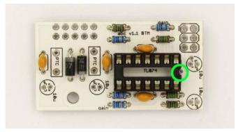
Now move to soldering the four 100nF ceramic capacitors (marked "104"). Then add the IC socket. Make sure that the notch on the socket matches the print on the board.
