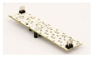
Solder the remaining **2x3 pin male header** on the top board.
