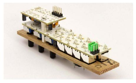
At last connect the boards back together and **install the jumpers** on the top board.
