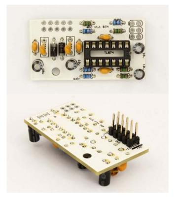
Next there are four **electrolytic capacitors**  $(10\mu F)$ . **Watch out for orientation!** There is a plus (+) sign on the PCB that should match the longer lead of the electrolytic capacitors. Then you add two **protective fuses** (marked "PTC" on board; be careful, they look quite similar to capacitors).
