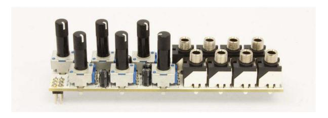
Place the spacer back in the opening. Take the **front panel**, screw and mount it with the board. Check that all the components came through. Secure the jacks to the panel with the **washers** and the **nuts** (keep in mind not to tighten the jack nuts too much as you may damage the panel!). Finally you are ready to solder the components
