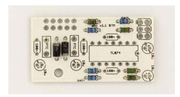
Insert and solder all 8 **resistors** (4x 100k, 2x 10k, 2x 1k). Then snip the leads as close to the PCB as you can (be sure to make this step on all remaining leads in the course of this guide). After that solder the two **diodes** (1N4007). Be careful, **diodes are polarized!** Make sure that the marking ring on the diode body matches the marking on the PCB.
