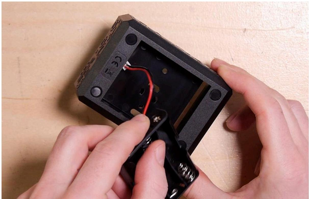
Connect the battery holder wire to the PCB, ensuring that the marked line on the plastic connector is facing upward. Gently bend the cable into the corner of the enclosure to prevent damage during assembly.
