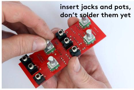
Place the **front panel** on and mount the pots and jacks with **nuts**. Check the position of all those components if they are flat on the board and solder them finally.
