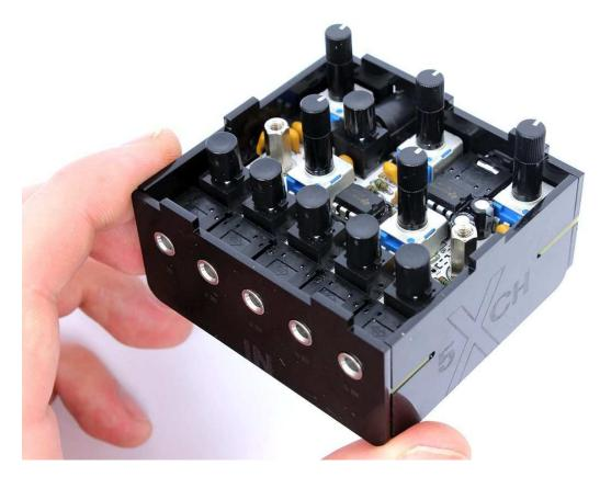
Finish the enclosure with the **top cover** and mounting the **screws**.
