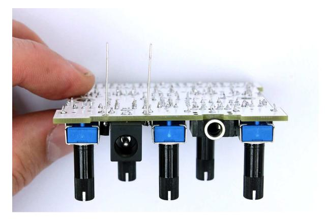
Let's secure the battery holder now with the **spacers** and **screws** (the longer ones) from the bottom. Watch out for the **orientation** of the holder!
