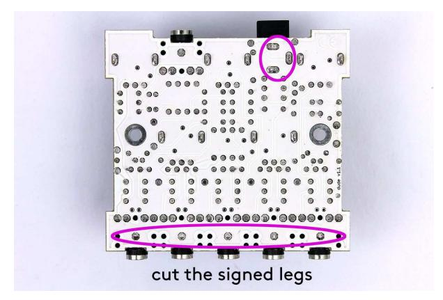
Take the remaining leads then and solder them into the holes near the power connector. It is good to melt some solder into the holes first and then reheat them and place the wire inside.
