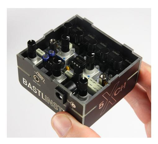
Finish the enclosure with the **top cover** and mounting screws.
