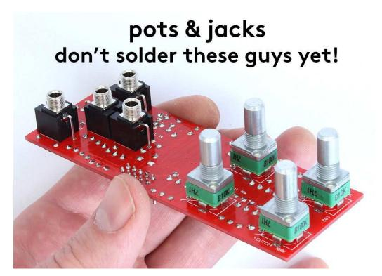
Place the **front panel** on and mount the pots and jacks with **nuts**. Check the position of all the parts if they are flat on the board and do the soldering.
