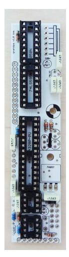
Next place and solder the sockets. Make sure that the notch is in the **same direction** as printed on the circuit board. The ATMEGA and MCP4921 circuit board prints have a little \* **orientation mark** instead of a notch. Both should be facing downwards.
