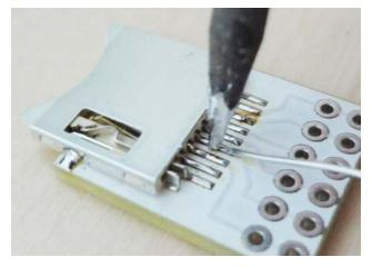
Alternatively you can apply some solder to all the pads before placing the card holder and then re heat them.
