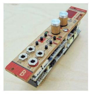
Before you connect anything, make sure that your system is disconnected from power. Also double check the polarity of the ribbon cable, the red cable should match the -12V rail both on the module and on the bus board!
