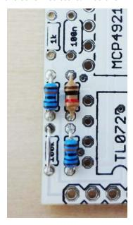
Next solder the power protection diode. Be careful though, diodes are **polarized!** Make sure that the marking ring on the diode body matches the marking on the circuit board.
