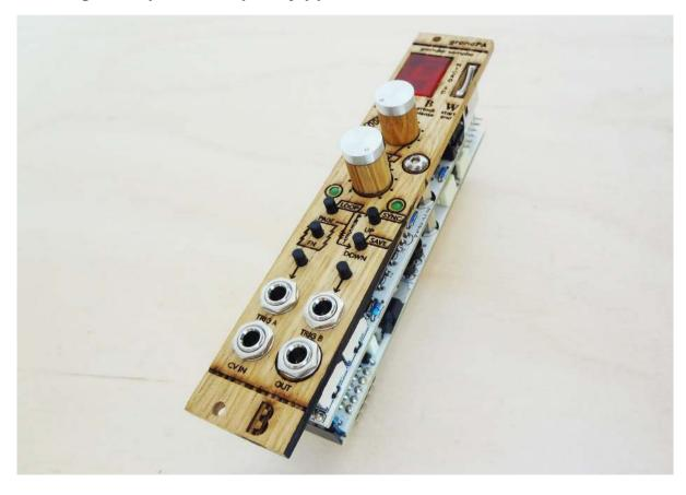
Before you connect anything, make sure that your system is disconnected from power. Also double check the polarity of the ribbon cable, the red cable should match the -12V rail both on the module and on the bus board!
