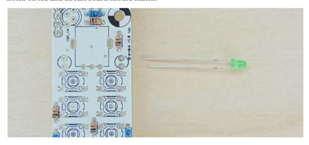
The RGB LED <u>long lead</u> should be in the third <u>hole</u> as well as the notches should match, like in the picture below. Still don't solder anything yet.
