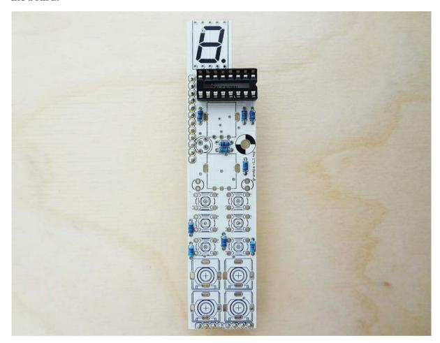
Then cut more of the breakaway headers and female headers at the right sizes, 12pins and 8pins. You will always loose one pin when cutting the female headers, so don't worry about it.
