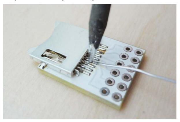
Alternatively you can apply some solder to all the pads before placing the card holder and then re heat them.
