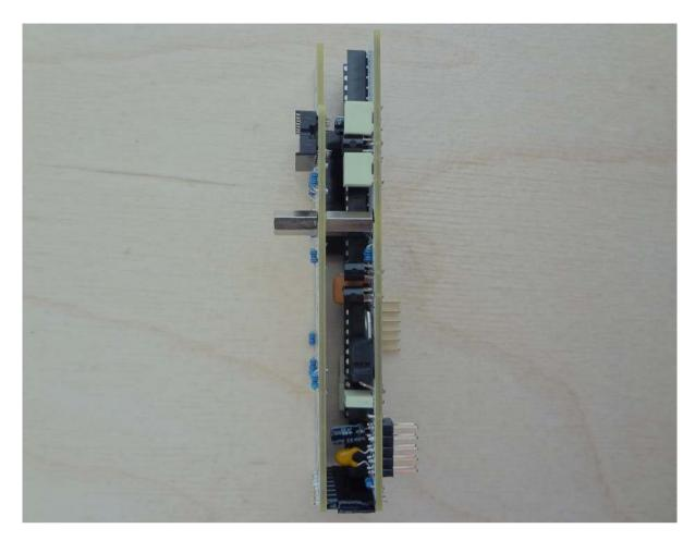
Also place the 74LS595 chip in it's socket. Make sure that it is <u>oriented properly!</u> The notches should match!
