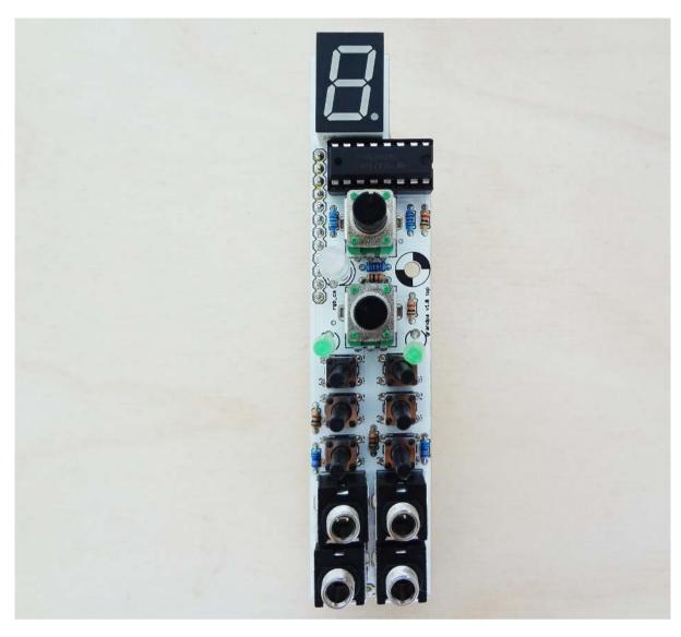
The LEDs are <u>polarized</u> so make sure that the <u>long leg</u> (+) is facing <u>upwards</u>. Also the notch on led and circuit board should match.
