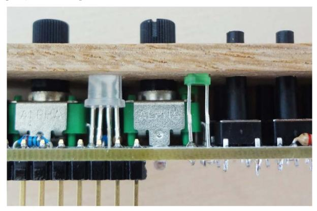
Also the display should be as close to the panel as possible.
