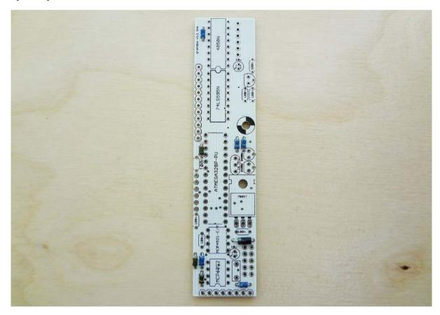
Next place and solder the sockets. Make sure that the notch is in the same direction as printed on the circuit board. The ATMEGA and MCP4921 circuit board prints have a little \* orientation mark instead of a notch. Both should be facing downwards. Then add the capacitors, there are seven 100n capacitors (marked 104). They might be in ceramic or polyester film package, don't worry they are not polarized.
