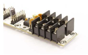
After the soldering don't forget to install the **nut with screw** on the voltage regulator and the **jumpers** (4x) into the default position.
