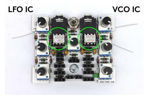
Bend the potentiometers legs on the edge of the PCB outwards (see the photo).
