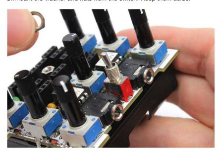
Now you can complete the Kastle with the plastic case parts. Start with the **side parts** (push them just in the corners). Finish it with the **top cover**, mounting the **nut** (to the switch) and **screw**. Again, please be gentle, you should not use too much power to put the parts together.
