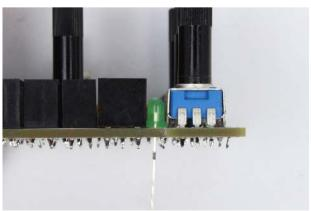
You will need the cutted leads from resistors now. Turn the PCB around and give a little bit iron into the remaining "HOLD", "BAT\_-" and "BAT\_+" holes. Re-heat them and insert the leads using needlenose pliers. The leads can not be connected with the potentiometers on the other side.
