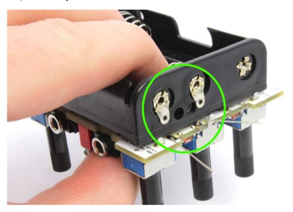
Mount the holder with **spacer** and the longer **screw**. It may be a little tricky. Don't tighten the screw too much because you are dealing with plastic material, you know.
