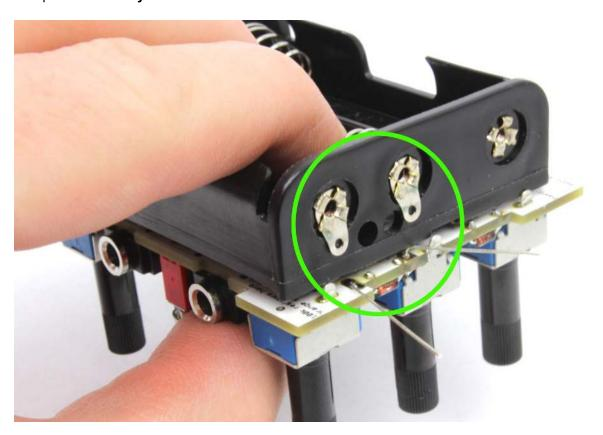
Mount the holder with **spacer** and the longer **screw**. It may be a little tricky. Don't tighten the screw too much because you are dealing with plastic material, you know.
