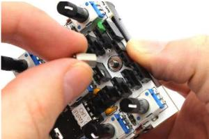
And now the last soldering challenge! You have to connect the leads with the lugs. **Do not let the lug heat too much!** (it would break the connection of the coil and the lug) Use just the tip of your soldering iron.
