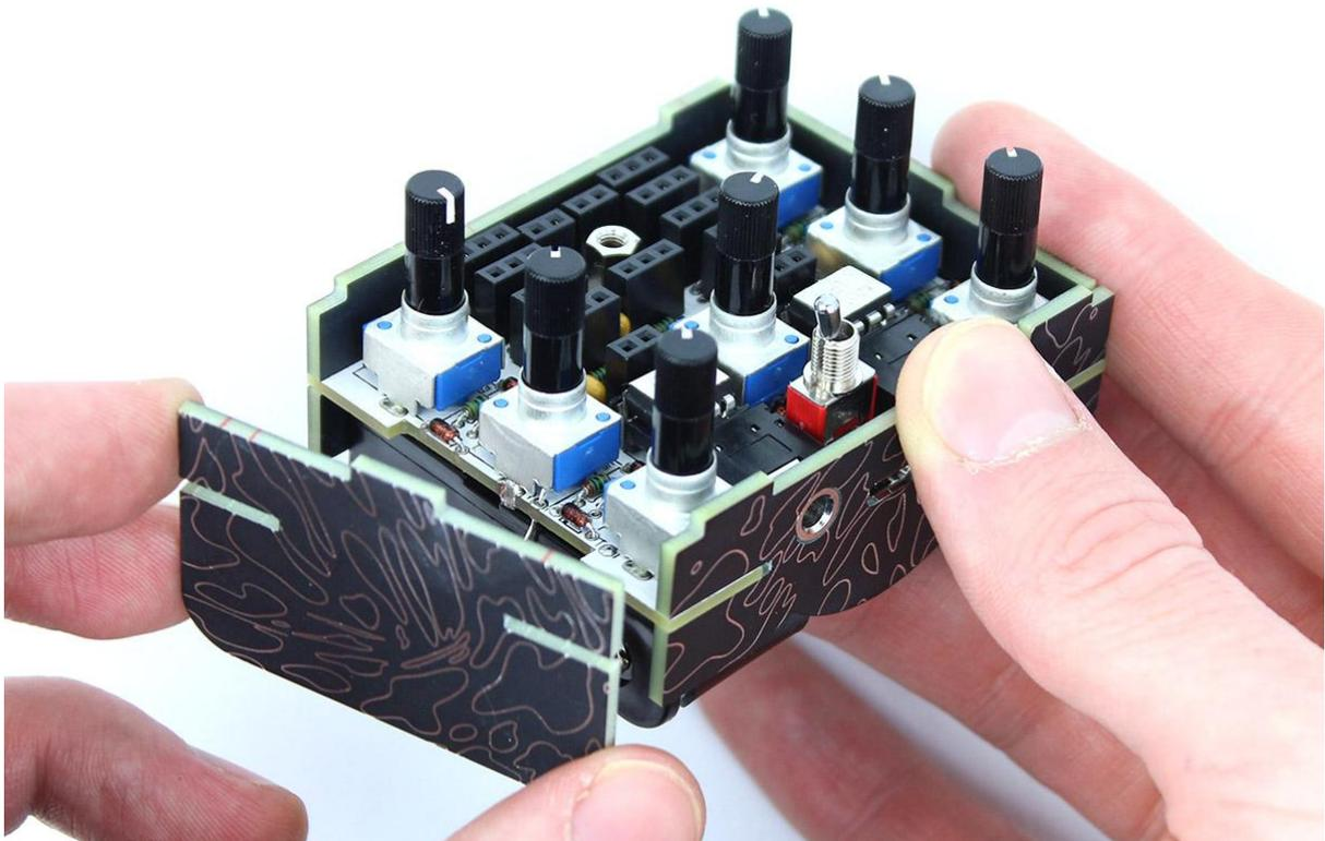
Finish it with the **top cover**, mounting the **nut** (to the switch) and **screw**.
