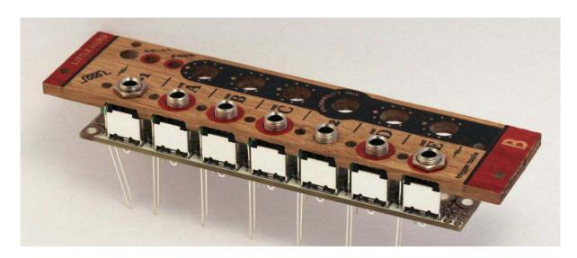
Then turn around this unit facing it with PCB upwards. Now push the LEDs leads to fit their heads on panel. **Make sure that everything is properly aligned**. Finally you are ready to solder all the components
