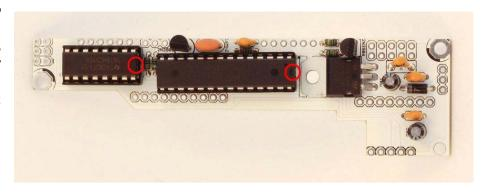
to place the ICs in the sockets (1x Atmega, 1x 74HC595). There is a notch on each IC that should match with the sign on the sockets. Check the picture.
