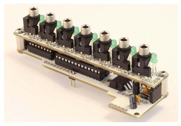
Now prepare two female headers (5 pin, 8 pin). Press it on pots board male headers and then take the two units, put them together (use the last screw for mounting) and solder the female headers on bottom board.
