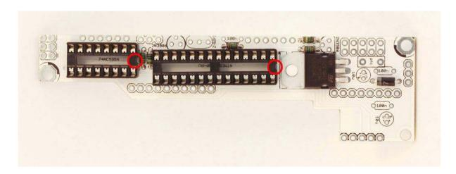
Now let's do some other parts. There are **three 100nF capacitors** (marked 104), **one protective fuse** (it looks quite similar to a ceramic capacitor but is placed in the "PTC" rectangular) and one **16MHz resonator** (the orange component with 3 leads). None of these parts are polarized so you can insert them in any direction.
