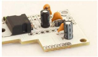
Now insert two transistors (2N3906). Again, watch out for orientation! Flat side of transistors must match the outline drawn on the PCB. You also want to push them closer to the PCB. Next don't forget
