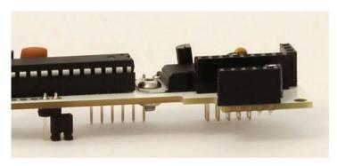
Congratulations! You have made it through, now just secure the jacks to the panel with **the washers and the nuts** (keep in mind not to tighten the jack nuts too much as you may damage the panel!), install two **jumpers** and a **screw with the small nut** on the voltage regulator (see the pictures).
