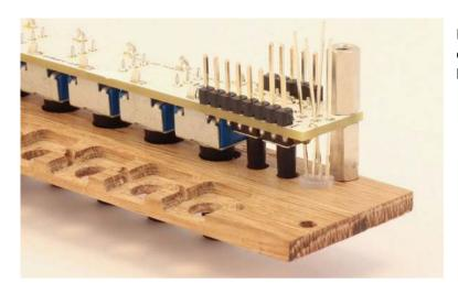
Push the LED leads to fit it's head on panel and solder it. You can keep the board on panel.
