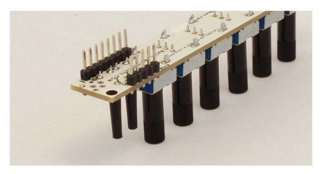
Now it is time to insert RGB LED. The longest lead should be in the third hole as well as the flat sides of the LED should match the printing. See the picture to check the orientation. Do not solder yet!
