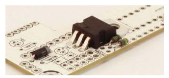
Next solder the **7805 voltage regulator.** Bend its legs as close to the body as possible, at a right angle to make sure that it lies flat on the circuit board.
