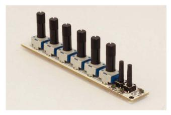
Take the **six potentiometers** and put them on the board. They have to sit right on the board and stand vertically. You can start soldering only one leg of each pot, then check the alignment and make an adjustment if needed. Solder the other legs. Then let's insert and solder **two small buttons**.
