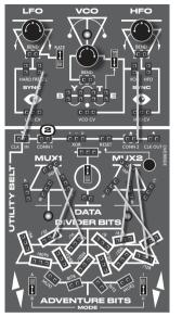
Safely patch signals from a modular synth into the bitRanger via the diode protected CV input and CONN jacks. Any signal above 5 volts will clip at 5 and below 0 volts will clip at 0.
