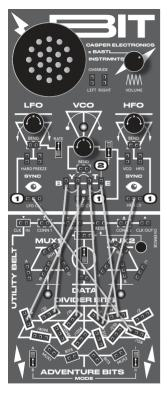
Use the bits as voltage sources to control the frequency of the three voltage controlled oscillators.
