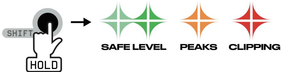
While holding the SHIFT button, the signal strength is indicated by the left light and when it reaches RED, it is clipping at the input, and you should lower your input gain (unless you want to go for that distortion 🤘). Keep the input gain so the signal is peaking into orange.
