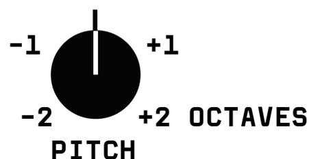
👉 🎛️ Hold the BANK button and turn the PITCH knob to change octaves. Each time the octave is adjusted, the sample is also triggered. For more details, refer to the [Quantizer](#) section.
