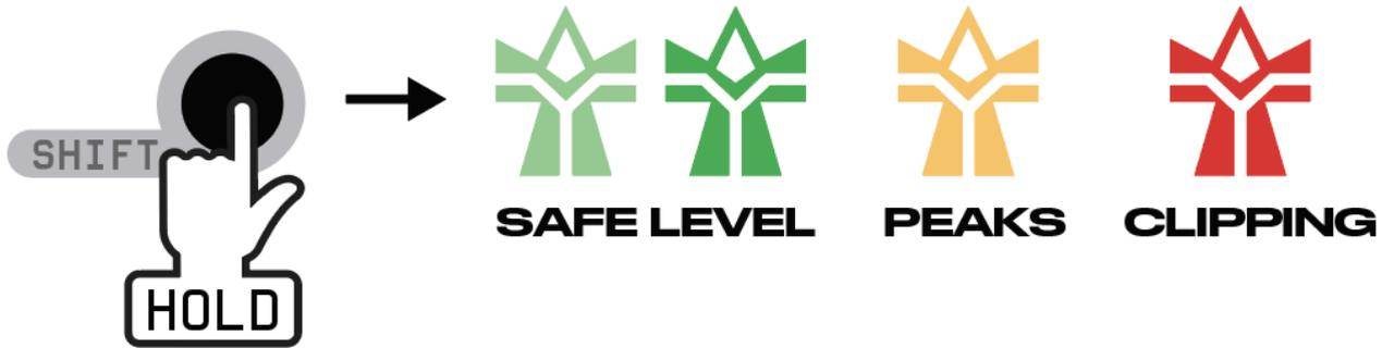
While holding the SHIFT button, the signal strength is indicated by the light in the word KASTLE and when it reaches RED, it is clipping at the input, and you should lower your input gain (unless you want to go for that distortion 🤘). Keep the input gain so the signal is peaking into orange.
