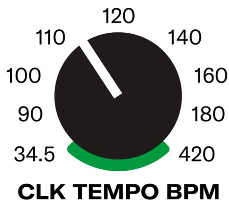
Hold REC and tap SHIFT to define the TAP Tempo (set the speed by tapping SHIFT). The final clock will be 4 times faster, assuming the clock is 16th notes and you are tapping quarter notes.
