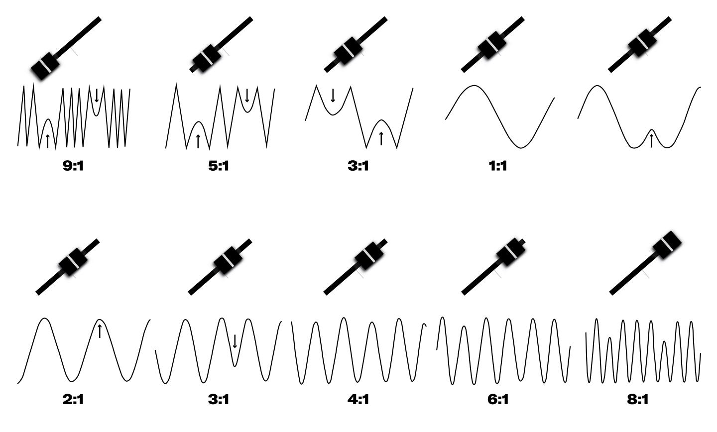
Ranges of both folding algorithms can be extended via CV or by assigning the CTRL knob to FOLD.
