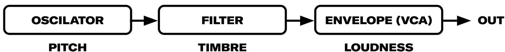
The deeper you delve into the SP2 architecture, the more clearly you will see the internal routing; and by fiddling with the MOD faders, you will uncover an unconventional synth-creature with unique behaviors. This architecture, including internal routings and normalizations, is illustrated on the front-facing side panel.
