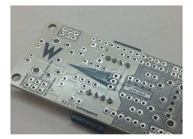
Step 3: Diode + resisotrs Now bend the legs of the diode 1N4148 and place where the picture shows the diode - the stripe (black on the diode) is the stripe (white in the print) - follow that polarity! Than 3 220 ohm resistors. Solder,cut, easy!
