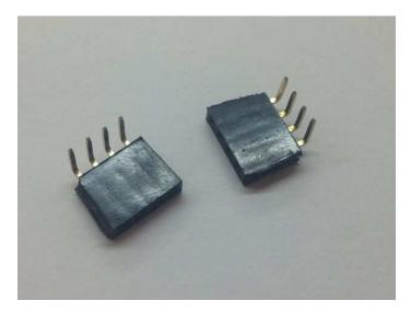
Step 2: Solder the 4-pin headers Lets start with soldering. All components solder from the component side of the board - the one with component labels. Place the headers and solder them - make sure they are straight.
