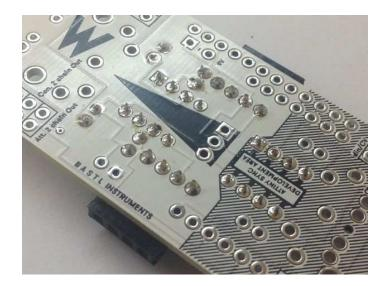
Step 4: 8 pin socket Lets place the 8 pin socket - follow its polarity (a little notch goes up). That is useful when inserting the ICs.
