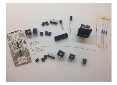
Step 1: Prepare the 4 pin angle female headers We need to make two 4-pin versions of angled female pin headers so we need to cut it. It is not possible to cut in between the pins so we always need to cut in the middle of another pin. Measure correctly and check the photos! When you have the 4 pins cut of the remaining plastic to be sure the headers would go nicely into the plastic housing later.
