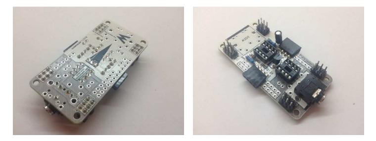
Step 8: Prepare the MIDI jack There might be not enough space if you have this type of MIDI jack with some plastic "left-overs" . Just cut them of and solder the connector. Leave no gap between the connector and the PCB.
