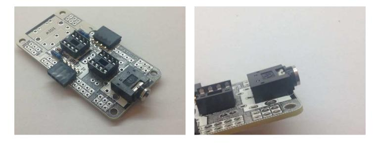
Step 6: Voltage regulator + capacitor Place these components and take care about the polarity. The regulator is indicated in the print. The capacitor short leg (-) goes closer to the pin header. (yes there is not so much space - will be improved in PCB 1.1 - doesn't affect functionality).
