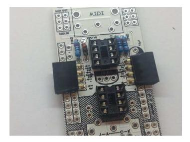
Step 5: Place the sync jack Place the sync jack - used for sync out. Make sure it is all the way down on the board and there is no gap between the jack and the board.
