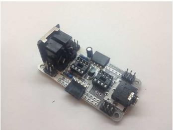
Step 9: Place the ICs The polarity or these ICs is indicated by a little dot in one corner of both ICs. Place them according to the picture. You might need to bend the legs a little bit so they would fit into the socket.
