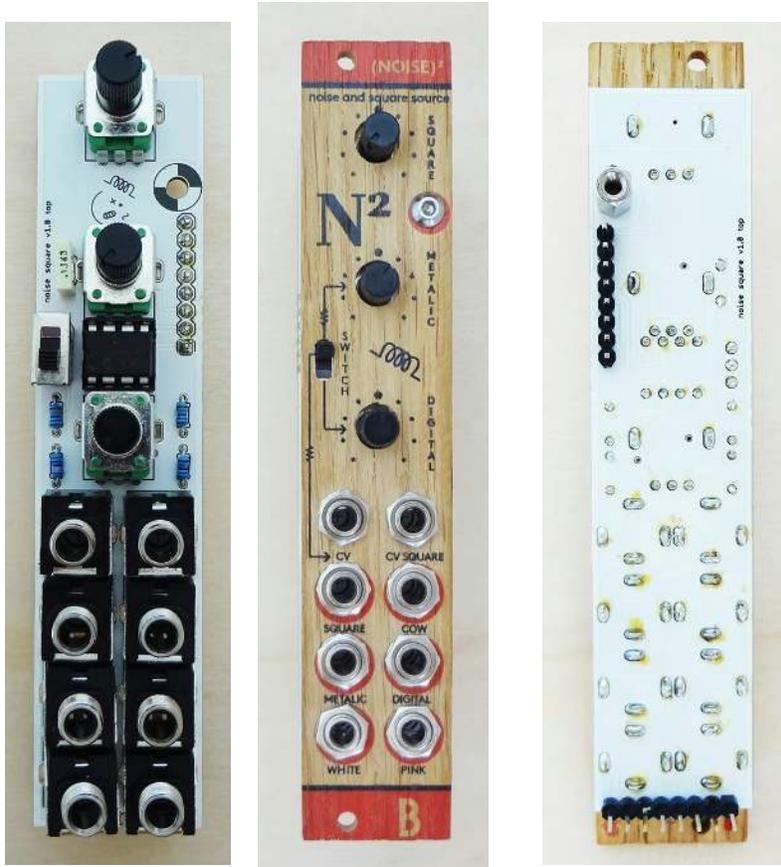
The switch **should have some space** off the board, or else it won't come through the panel, like in the image below. Solder the switch and the rest of the components.
