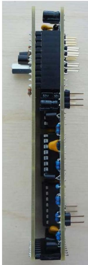
Now to ensure that the headers are properly aligned, screw the hex screw and the standoff on bottom board. Place the female headers on button board with the male pins inserted. Now place top board, screw with the standoff screw and finally, solder the headers to both boards. Just like in the image below.
