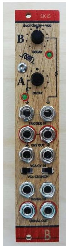
The switch and the LED **should have some space** off the board, or else they won't come through the panel, like in the image below. Solder the LEDs, the switches and the rest of the components.
