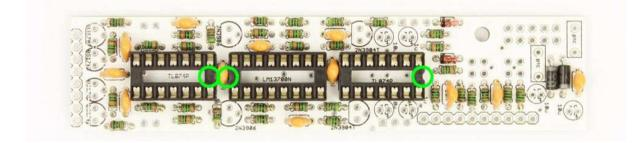
Next solder in the **transistors** (be careful though, they look quite similar): two **2N3904**, two **2N3906** and four **BS170**. Take care that they are oriented the same way as printed on the board. Flat side of transistors must match the outline drawn on the PCB.
