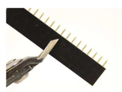
Prepare pinheaders with your flush cutters now. You need one **8 pin male** and **10 pin male**. Also do the same lengths from the **female** pinheader (you will always lose one pin when cutting the female headers, so be sure to cut it always after the last required pin - check the picture to see where to cut to get 8 pin).
