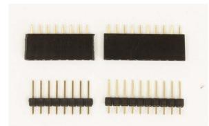
Now to ensure that the headers are properly aligned, screw the hex screw and the standoff on the bottom board. Place the female headers on the bottom board with the male pins inserted. Now place top board, screw with the standoff screw and finally, **solder the headers to both boards**. Unscrew the top sacer and disconnect the boards then.
