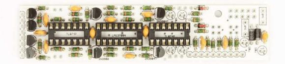
Turn around the PCB. Prepare with your flush cutters and solder the following **pinheaders**:
