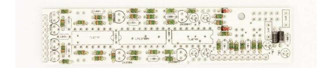
Now move to soldering the IC sockets (2x 14 pin, 1x 16 pin). Make sure that the notch on the socket matches the print on the board. After that add some capacitors. There are eight 100nF (marked "104") and four 10nF (marked "103").
