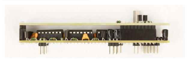
Place the two **potentiometers** to their respected places on the board. Push them well until they sit absolutely flat on the board, but don't solder them yet. Next, place the mono **jacks** (10x) on the board, the **LEDs** (2x) and the **switches** (2x). The **LEDs are polarized** so make sure that the longer leg matches the plus hole (+). Also the flat side on LED and the PCB should match. **Still don't solder anything yet**.
