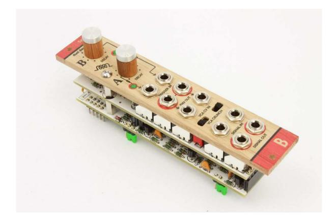
Before you connect anything, make sure that your system is disconnected from power. Also double check the polarity of the ribbon cable, the red cable should match the -12V rail both on the module and on the bus board!
