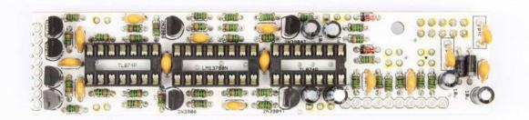
Next don't forget to place three **ICs** into the sockets (1x LM13700N, 2x TL074). There is a **notch** on the ICs that should match with the notch on the socket.
