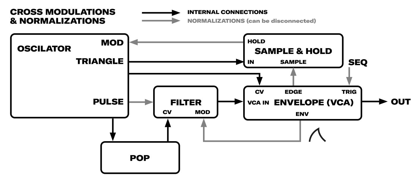
Normalizations are pre-made connections within the instrument that can be interrupted by plugging new signals into the dedicated normalization jacks. These jacks are marked with arrows showing the signal that is normalized to the jack.
