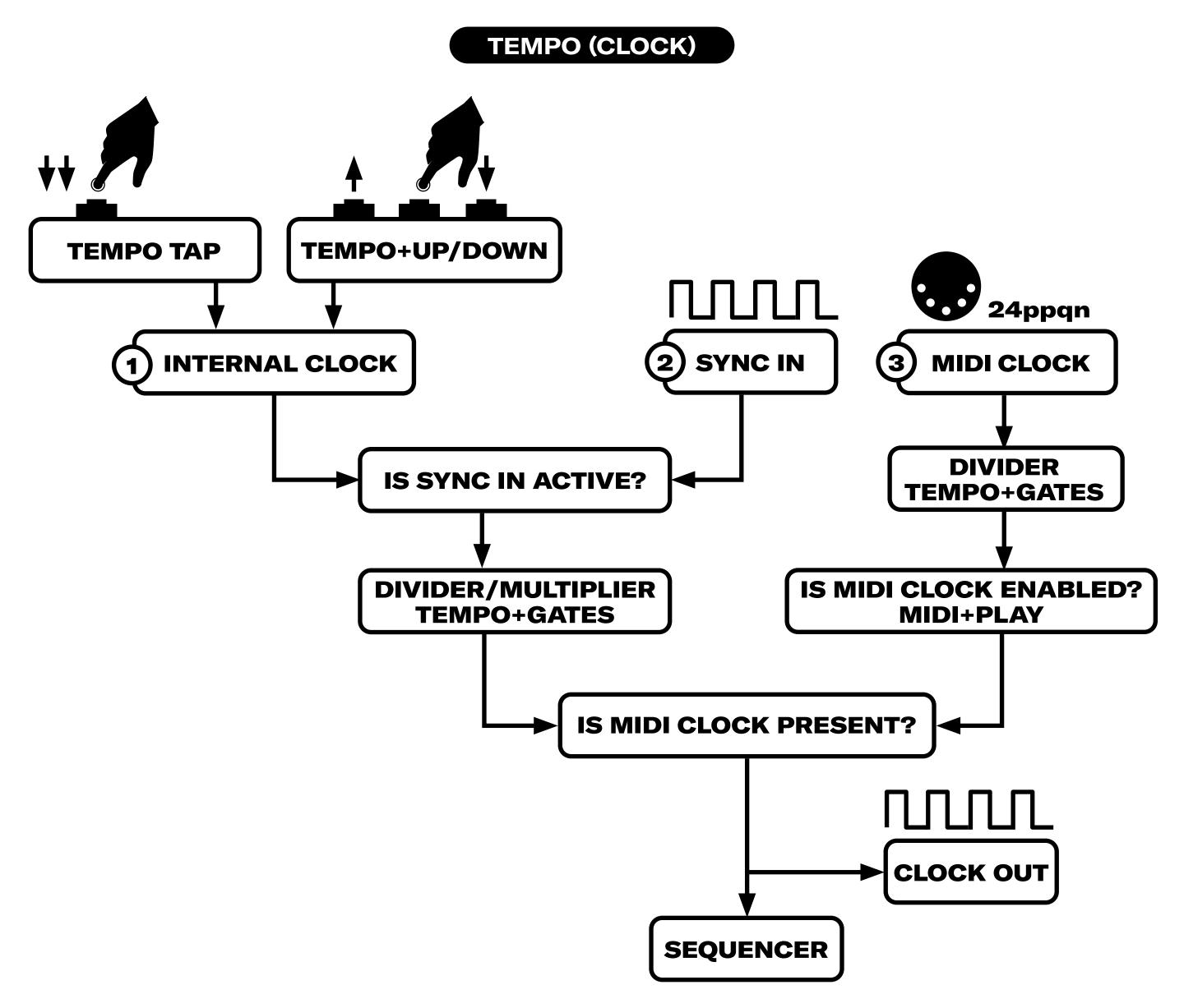
Hold the MIDI button and press PLAY to enable/disable the MIDI clock (indicated by the PLAY light). Use TEMPO+GATES to select a divider to the tempo, at which the sequencer will be clocked.
