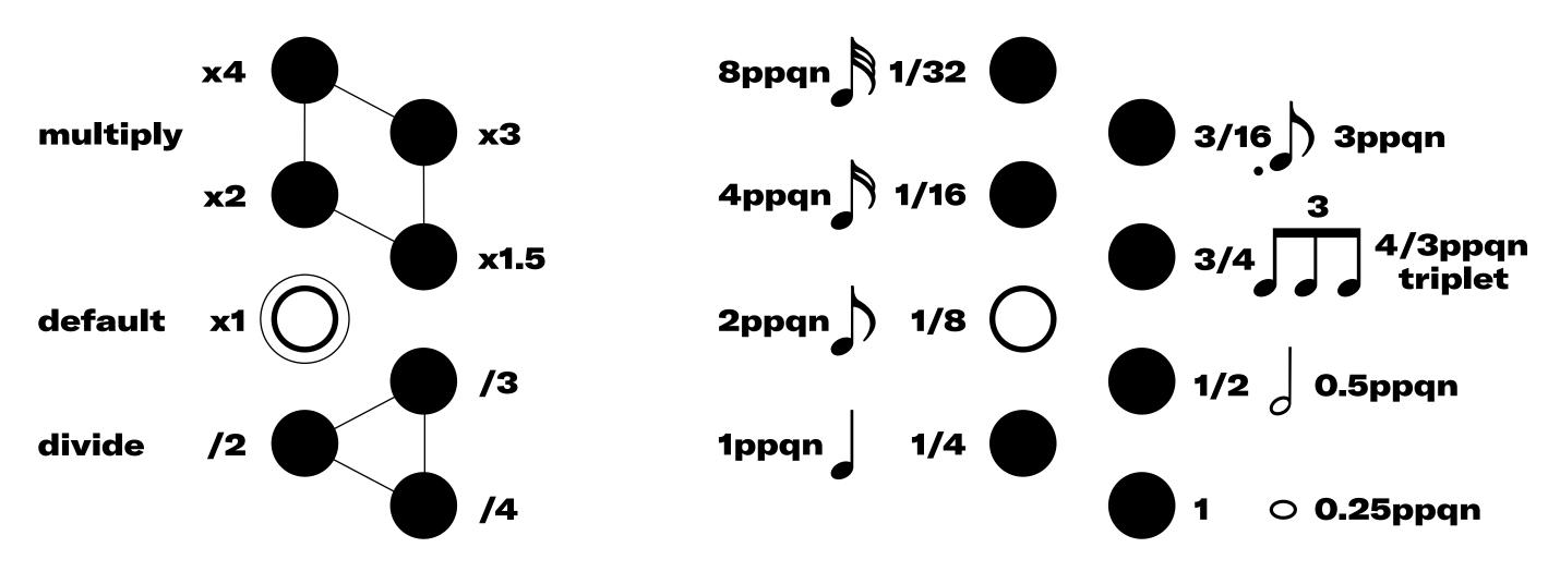
The divider on GATE 5 is the default for both clocking options. Use it when unsure.
