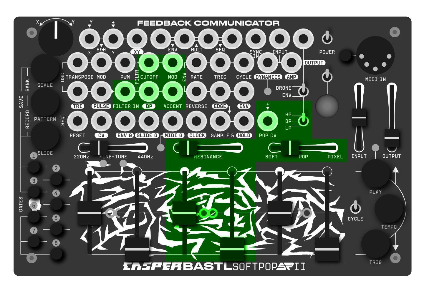
The filter is the main timbral shaping tool on the Softpop. You can use it to take away specific frequencies and harmonics while accentuating others. You can also animate that process and create the iconic filter sweep. Softpop's filter is also a unique sound source: it is optimized for extended filter techniques such as overdriving, pinging, self-oscillation, or filter FM.
