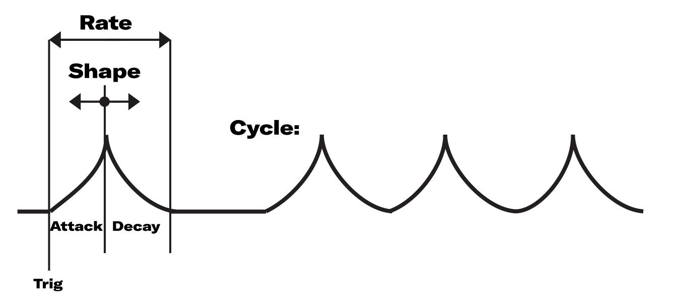
The SP2's envelope is very flexible when it comes to voltage control. Use the RATE input to control the RATE parameter or send gates to the REVERSE input to invert the proportion of attack and decay times set by the SHAPE fader. You can also activate cycling by a high gate on the CYCLE input.
