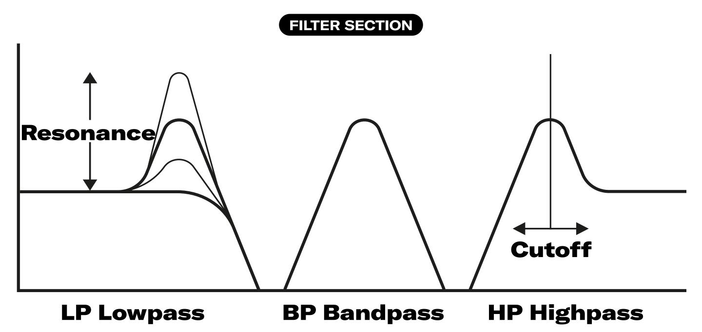
RESONANCE fader sets how much the CUTOFF frequency is emphasized. It creates a resonant peak in the spectrum, and when pushed even further, it will make the filter ring out (pinging technique) or even self-oscillate.
