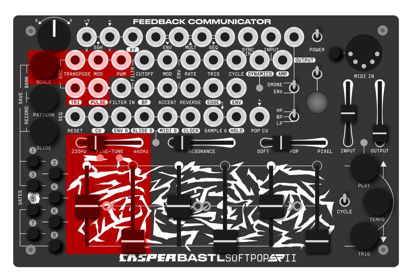
The oscillator is Softpop's source of tonality. It is either an analog oscillator that is digitally analyzed and controlled or a fully digital oscillator. This manual describes the digital oscillator functionality. For more information on the analog oscillator functionality, see the respective manual <a href="https://example.com/here/">here</a>.
