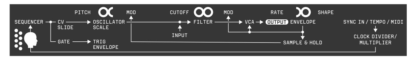
The envelope is normalized to the CUTOFF MOD, so you can use it to control the timbre of the filter by bringing up the CUTOFF MOD fader.
