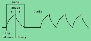
TRIG will trigger the envelope once. The DRONE/ENV switch lets you select between DRONE (sound always on) or ENV (volume increases with the envelope).
