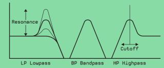
The HP/BP/LP switch selects the filter type. HP=Highpass: passes frequencies above cutoff (cuts bass)
