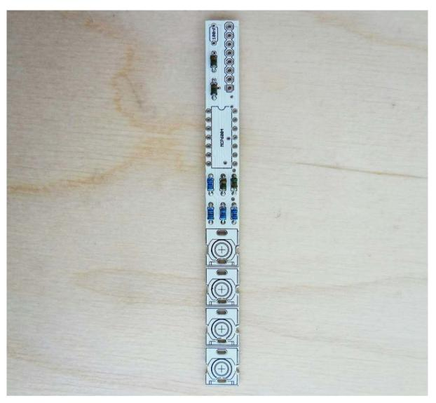
Next place and solder the socket. Make sure that the notch is in the **same direction** as printed on the circuit board.
