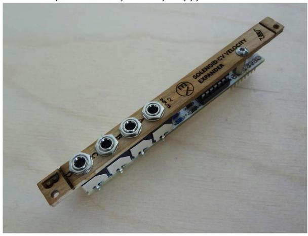
Before you connect anything, make sure that your system is disconnected from power. Also make sure that cable connections on both modules are in the same side.
