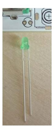
The LED is **polarized** so make sure that the long leg (+) is facing upwards. Also the notch on led and circuit board should match. Still don't solder anything yet.
