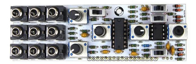
6) Place the **front panel** on the top board and mount the jacks.
