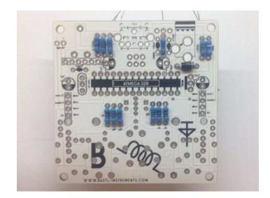
Step 2: Place the protective diode Care of the polarity indicated by the stripe
