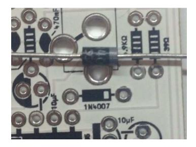
Step 3: Solder Bend the legs or the components slightly and turn the board upside down and solder each connection properly. Than cut the legs.
