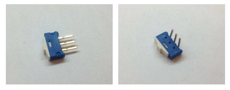
Step 7: Capacitors, Resonator Regulator Switch Power Jack IMPORTANT: in version 1.1 with full plastic housing the switch has to go from the other side of the board ! as on the pictures !
