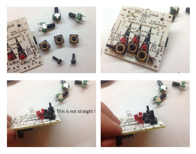
Step 13: Knobs For left and right knob it is easy to place them and solder them. The top knob needs a bit of adjustment so it fits. Make sure the knobs are soldered straight and as close to the pcb ad its construction allows. Otherwise the PCB might not fit correctly into the housing !!! The volume knob might also need a bit of adjustment so it fits the holes. (only for version 1.0)
