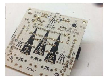
Step 8: FTDi Break Out Connecor- The Hack Port Solder the 6 pin bent header on the right place. To hold it in the place put something like pliers underneath.
