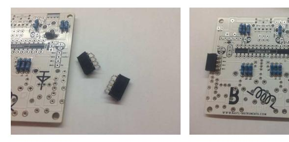
Step 5: Atmega Socket and Audio Jack On the chip socket mind the polarity indicated by the notch. On the audio connector try to solder it the way that there is NO gap between the connector and the pcb. Than cu the remaining legs of the jack. Double check that you solder from the correct side of the pcb!
