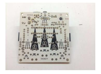
Step 10: Leds The leds have polarity indicated on the board. The longest leg of the led is + The RGB led goes as deep as the stoppers on its legs are.
