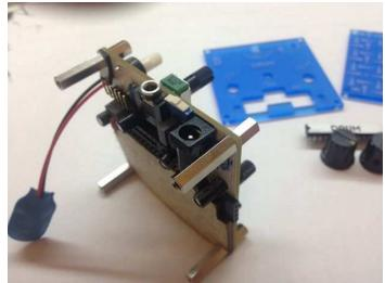
Step 17: Place The Chip Follow the polarity indicated by the notch of the socket.
