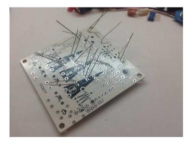
Step 9: Interface Side The component side is ready so lets solder from the Interface side.
