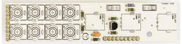
Insert now all the other parts (jack connectors, potentiometers, switches and LED) but do not solder them yet:
