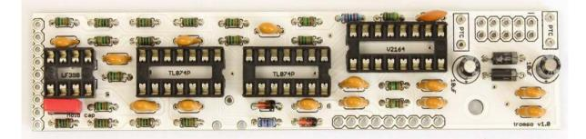
Turn around the PCB to solder the **2x5 pin male header** and solder it. Be careful to solder the headers straight. You may first solder one of the pin, take the board in your hand and re-heat that pin while you are adjusting the header straight. Add also the **trimmer**.
