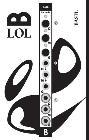
LOL is a performative 3 channel passive mute module with latching push buttons, LED indication, and normalization between inputs. It is intended to be a small and low-cost mute, but it can also be used as a switched multiple. LOL has 3 channels: O, M and G. Each channel consists of an INPUT, a MUTE **BUTTON** with an LED, and an OUTPUT.
