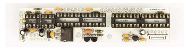
Again turn around the PCB and insert and solder next male pinheaders: one 6 pin and one 2x5 pin. From the other side solder the 1x6 pin right angle. Again you should be careful to solder the pinheaders straight and flat with the board.
