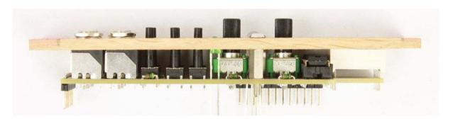
Turn over the board and clip off the leads of the jacks as they might short the capacitor.
