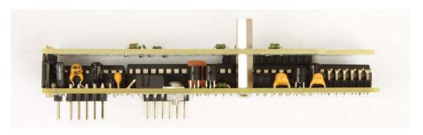
Place the two **potentiometers** to their respected places on the bottom board. Push them well until they **sit absolutely flat** on the board and solder them. Next place the **IC socket** (watch out for
