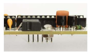
Place the **ICs** into the sockets (Atmega, 74HC595, CD4050BE, MCP4921, MCP6002). There is a notch on each IC that should match with the sign on the sockets. Check the picture.
