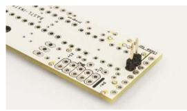
Turn around the PCB and prepare one **2 pin male** header with your flush cutters. First solder in just one of the pins, then take the board in your hand and re-heat that pin while pressing down on the header to align it (be careful though, you don't want to touch the pin you are heating up) wait for it to cool and solder the rest of the pins.)
