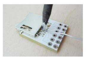
Now it's time for a little challenge. Solder the SD card holder to its little board. It is SMD component but don't let that scare you, it's pretty simple. A fine tip soldering iron is suggested here.
