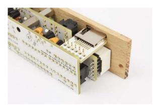
Place the SD board on the 6 pin male, connect the boards and solder it.
