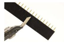
Prepare pinheaders with your flush cutters now. You need one **8 pin male** and **12 pin male**. Also do the same lengths from the **female** pinheader (you will always lose one pin when cutting the female headers, so be sure to cut it always after the last required pin - check the picture to see where to cut to get 8 pin).
