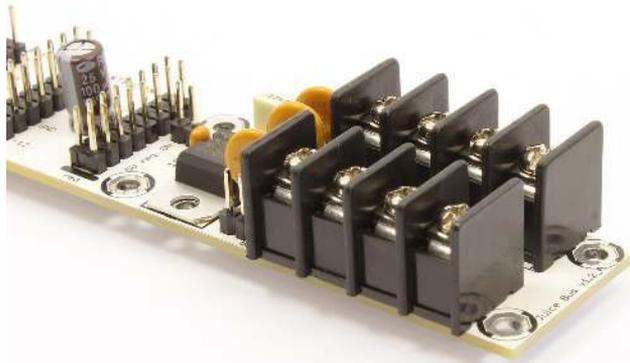
After the soldering don't forget to install the **nut with screw** on the voltage regulator and the **jumper** (4x) into the default position.
