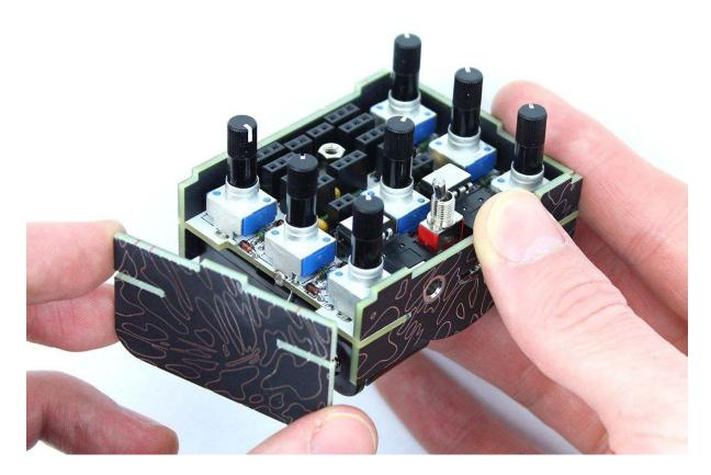
Finish it with the **top cover**, mounting the **nut** (to the switch) and **screw**.
