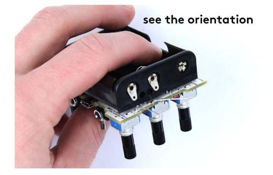
Mount the holder with **spacer** and the longer **screw**. It may be a little tricky. Don't tighten the screw too much because you are dealing with plastic material, you know.
