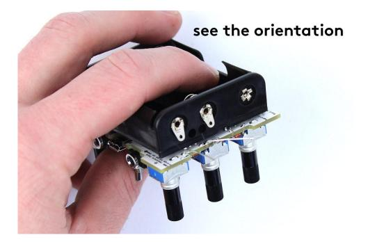
Mount the holder with **spacer** and the longer **screw**. It may be a little tricky. Don't tighten the screw too much because you are dealing with plastic material, you know.
