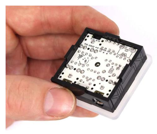
Finish the mounting by placing the **bottom cover** and securing it by the **screw**.
