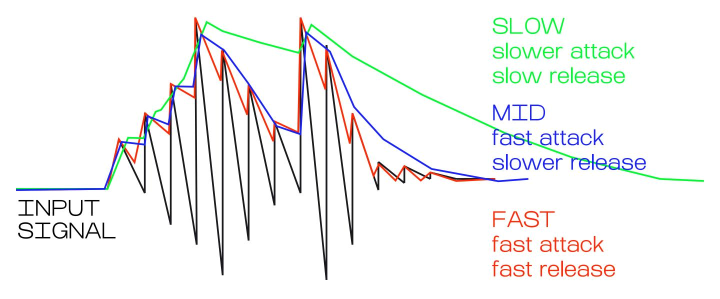
Tip: Send triggers to SIDE CHAIN IN and use the SIDE CHAIN switch to get different envelopes. Use these envelopes for compression or use them independently.
