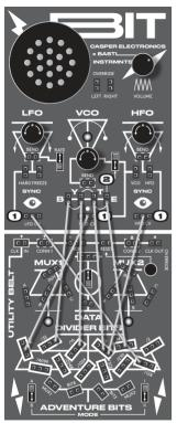
Use the bits as voltage sources to control the frequency of the three voltage controlled oscillators.
