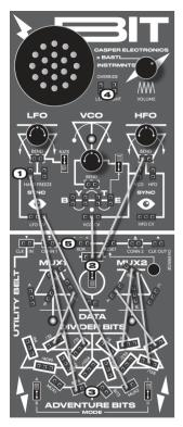
Patching techniques for the adventurous user. These features are most effective when integrated into complex patches that incorporate the MUX1&2 sections and CV sockets.
