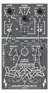
Safely patch signals from a modular synth into the bitRanger via the diode protected CV input and CONN jacks. Any signal above 5 volts will clip at 5 and below 0 volts will clip at 0.
