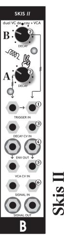
Skis II is a dual voltage controlled decay envelope with a dual VCA. Both envelopes and VCAs are normalised, but they can be used independently. The decay envelopes are exponential and they can also be set up as release envelopes. Both VCAs are linear. A typical application of Skis is to take two signals (noises, for example) and generate percussive sounds with adjustable DECAY from them with a TRIGGER signal.
