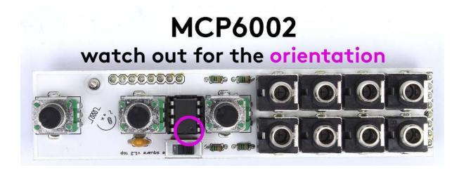
Congratulations! You have made it through. Now just connect the boards, add the knobs and your NOISE SQUARE is ready to go! Before you connect anything, make sure that your system is disconnected from power. Also double check the polarity of the ribbon cable, the red cable should match the -12V rail both on the module and on the bus board!
