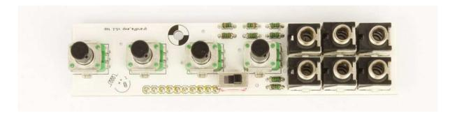
Place the **spacer** back in the opening. Take the **front panel**, **screw** and mount it with the board. Check that all the components came through. Secure the jacks to the panel with the **washers** and the **nuts** (keep in mind not to tighten the jack nuts too much as you may damage the panel!).
