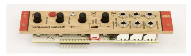
Push the **switches** to be sure that they come through the panel. Make sure that everything is properly aligned. Now you are finally ready to solder all these components.
