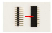
To ensure that the headers are properly aligned, screw the hex screw and the 11 mm spacer (nut - nut) on bottom board. Place the female headers on bottom board with the male pins inserted. Connect the boards together and mount them with the other spacer (10 mm one, screw - nut). Now you can solder the headers on both boards.
