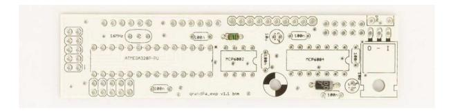
Next place and solder the **IC sockets** (8 pin, 14 pin and 28 pin). **Notice the notch** on them. Make sure that it is in the same direction as the printing on the board (the sockets are all oriented the same way).
