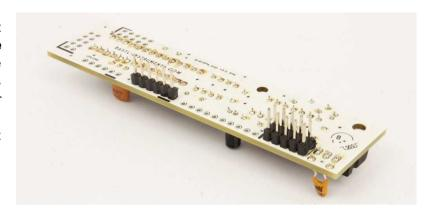
Now you can insert three **ICs** into the sockets (MCP6002, MCP6004, Atmega). **Watch out for orientation!** There is a notch on the ICs that should match with the notch on the sockets. Install also the **small nut** and **screw** on the voltage regulator.
