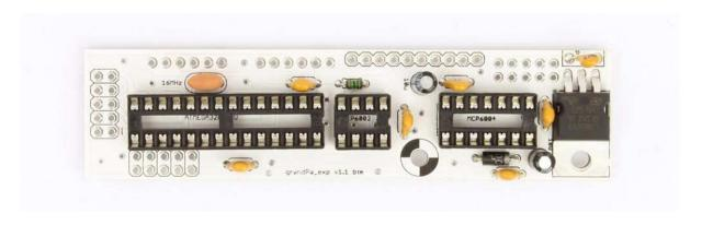
Turn around the PCB and insert and solder the **male pinheaders** (6 pin, 2x5 pin). Be careful to solder the pinheaders straight! You may first solder one of the pin, then take the board in your hand and re-heat that pin while pressing down on the header to align it. Wait for it to cool and solder the rest of the pins.
