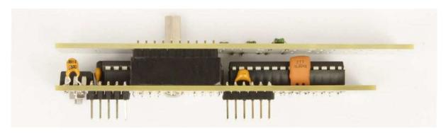
Unscrew the spacer on top and disconnect the two boards. Next place the four **potentiometers** (B100k) to their respected places on the top board. Push them well until they sit absolutely flat on the board. Then place the **mono jacks** and the **switch** on the board. **Don't solder anything yet**.
